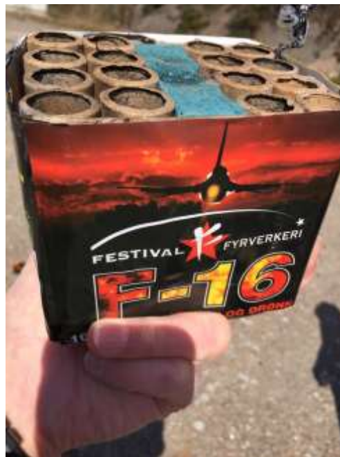
Figure 3 - Product collected by the Norway - all the shots failed to fire correctly.
