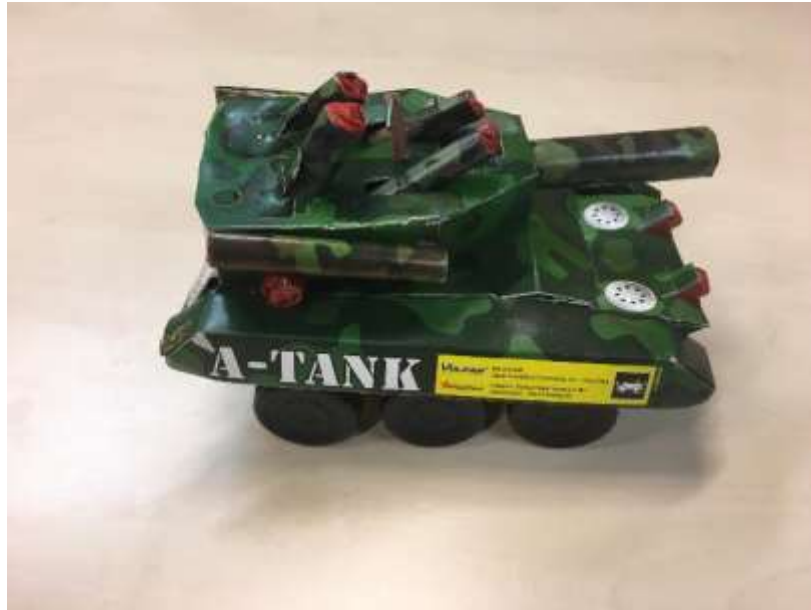
Figure 7 - Shows sample BE 116 - A Ground Mover which has been modelled in the form of a toy, in this case a tank
