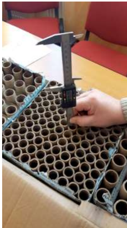
Figure 6 - Sample SL 13 - Compound firework in which this part of the firework failed to fire correctly.
