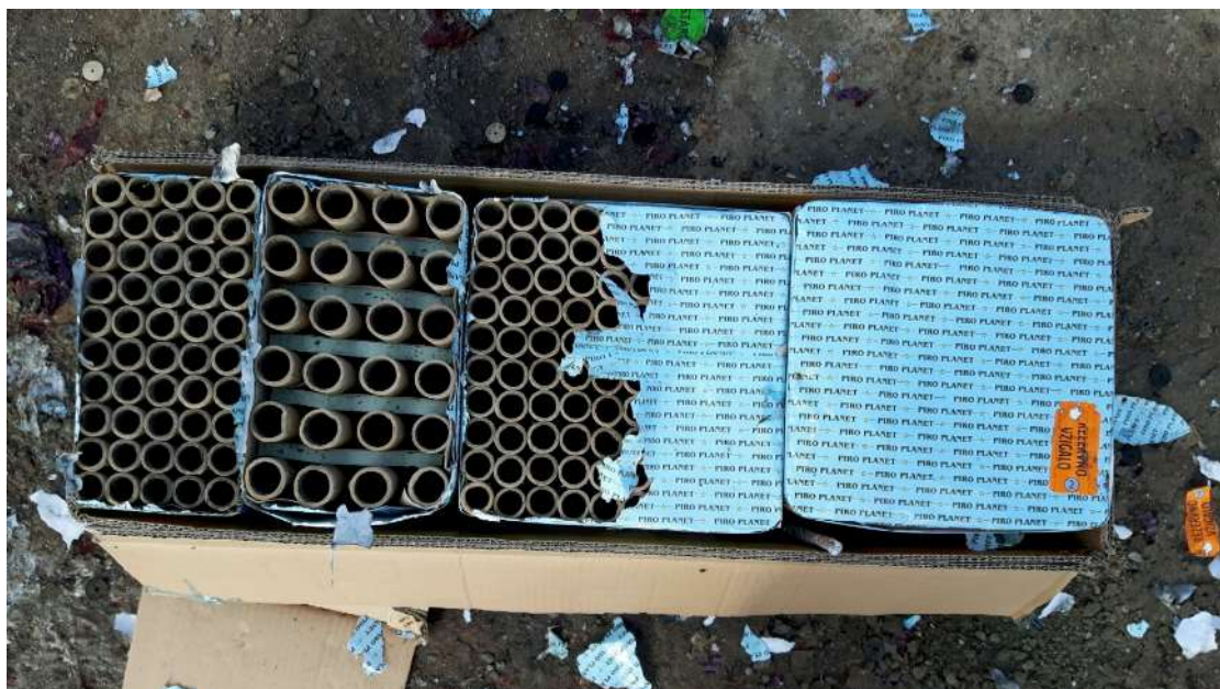
Figure 4 - A further example of samples SL 13 showing the parts that failed to fire.
