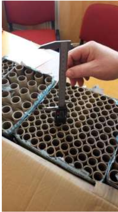
Figure 5 - Sample SL 13 - Compound firework showing that in this part of the firework the tube fired correctly
