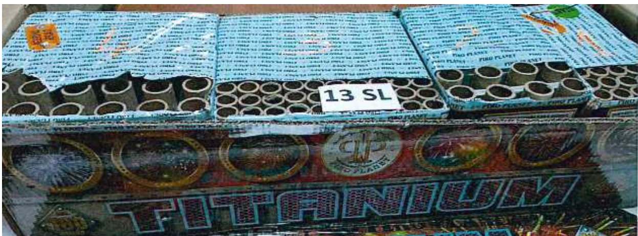
Figure 1 - Product 13SL - An example of a compound firework
