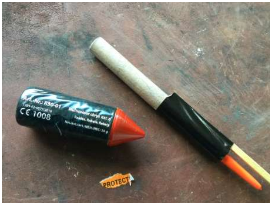
Figure 9 - Rocket in which the plastic fuse cover precluded access to the fuse and in which the head of the rocket became detached when the lab staff attempted to remove the fuse cover.
